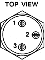
1 SOURCE 2 GATE 3 DRAIN
